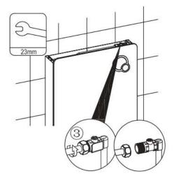
Disconnect the hose from the shut-off valve
